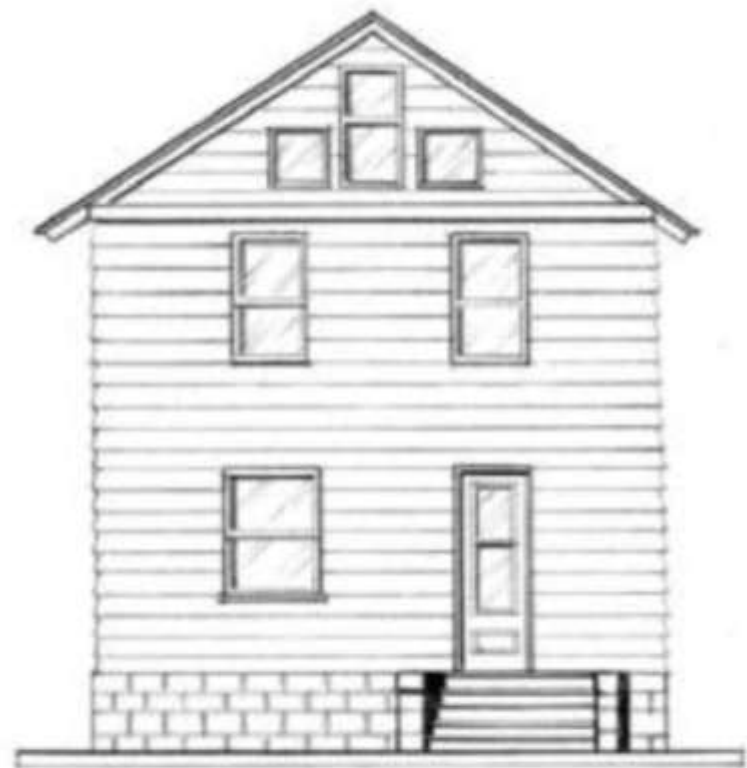
Inappropriate remodeling; the porch and trim have been removed and artificial siding of the wrong dimension has been added
